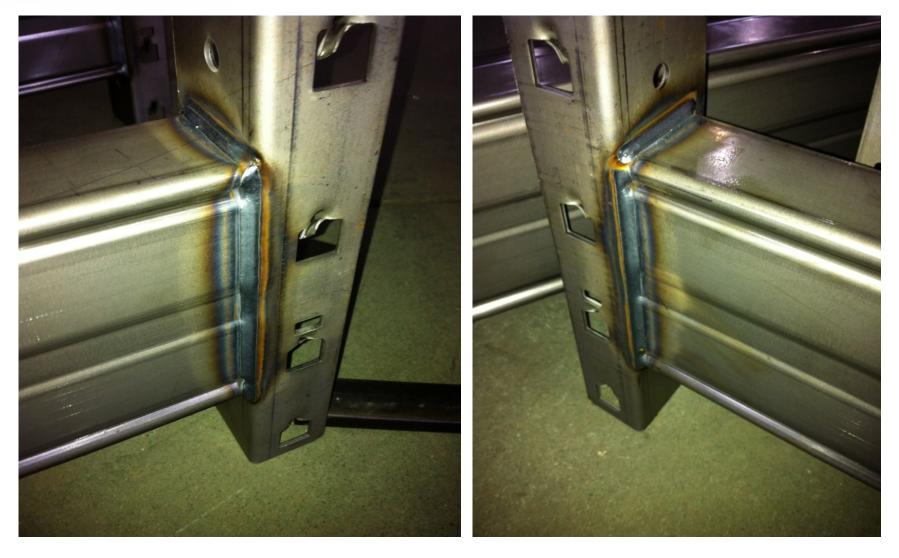
This machine can weld Step Beam, Box Beam, C Channel Beam etc, welding 2 sides, 3 sides and 4 sides. 60 to 90PCS per hour. Operation Video: <u>https://youtu.be/yroxNx6vCzl</u>
